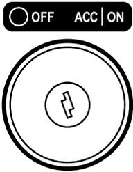
The key switch controls the motor and electrical system. A key is used to select the key switch position. The key can only be inserted or removed when the key switch set to OFF.
